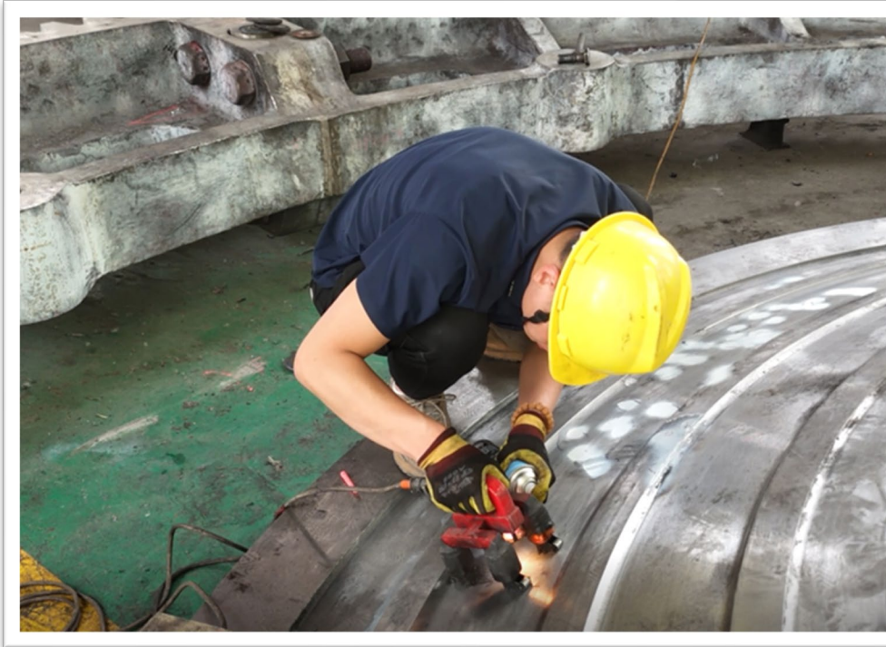
Magnetic Particle Testing (MT)
